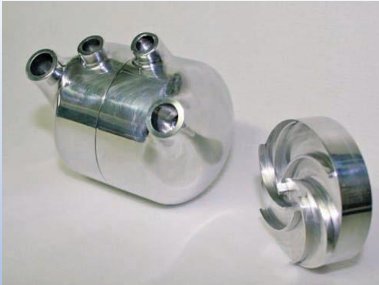
FIGURE 62-15 The BiVACOR total artificial heart employs a single moving part—a central magnetically levitated rotor—to provide complete cardiopulmonary support. (Reproduced, with permission, from BiVACOR, Inc.)
